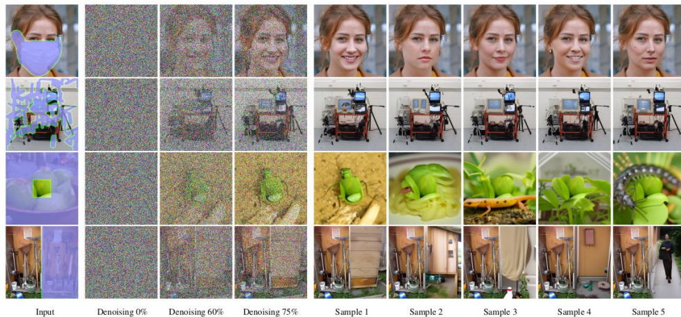
Figure 1. We use Denoising Diffusion Probabilistic Models (DDPM) for inpainting. The process is conditioned on the masked input (left). It starts from a random Gaussian noise sample that is iteratively denoised until it produces a high-quality output. Since this process is stochastic, we can sample multiple diverse outputs. The DDPM prior forces a harmonized image, is able to reproduce texture from other regions, and inpaint semantically meaningful content.
